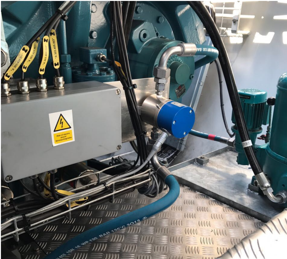
Bypass sensor installation, Siemens 3.2 WT
